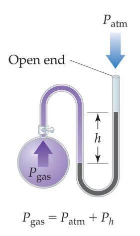
This device is used to measure the difference in pressure between atmospheric pressure and that of a gas in a vessel.
